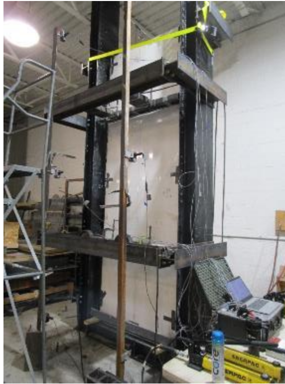
Photo No. 2 Transverse Load Test Setup - Loaded Side
