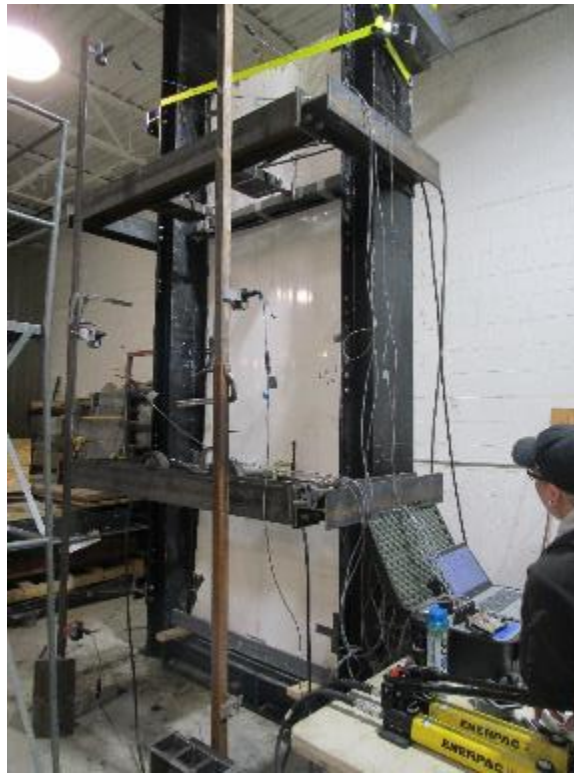
Photo No. 4 Transverse Load Test Under Load
