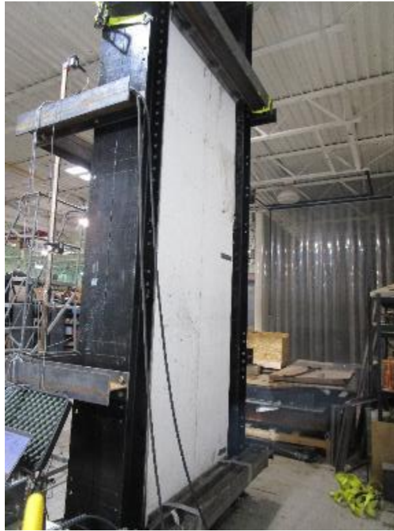
Photo No. 3 Transverse Load Test Setup - Support Side
