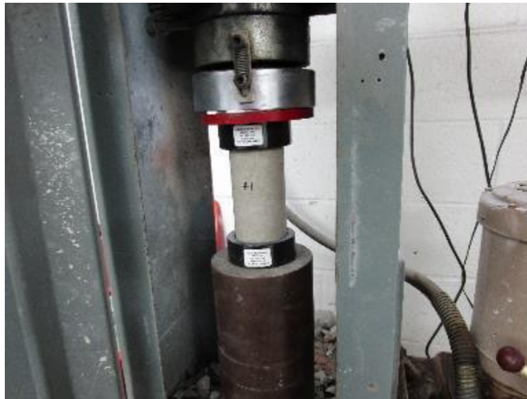
Photo No. 7 Concrete Cylinder Compression Testing Setup
