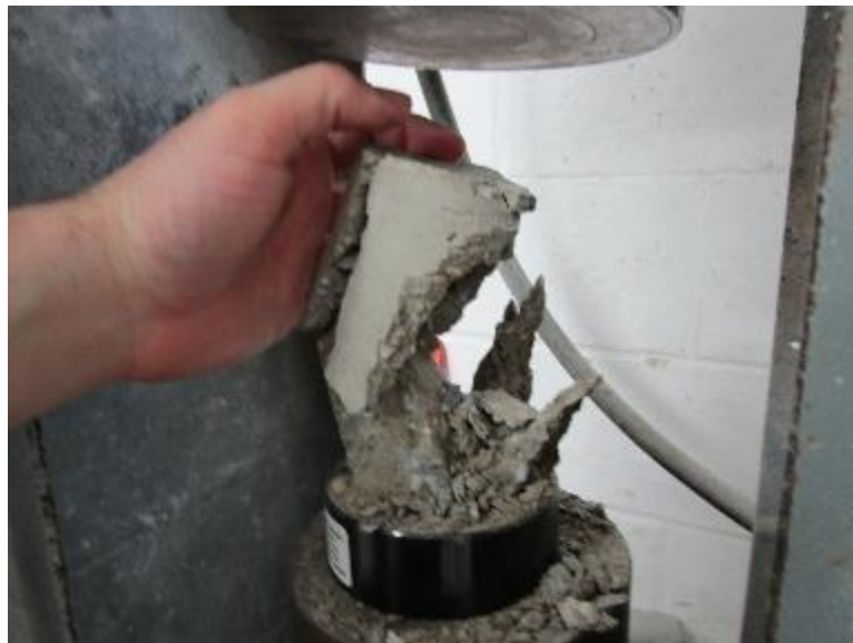
Photo No. 8 Concrete Cylinder Compression Testing Failure
