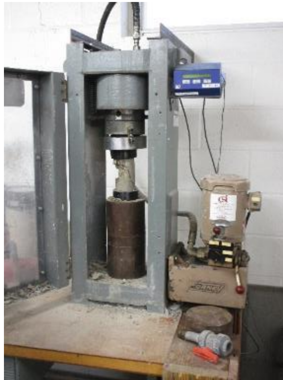
Photo No. 3 Concrete Cylinder Compression Testing Failure
